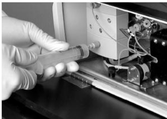
Figure 3-11: Purging Air from the Check Valves
